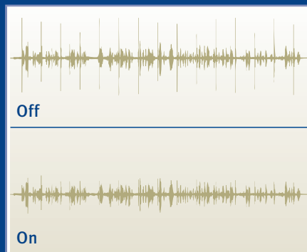
Speech + shock when antiShock-Off (top) and antiShock-On (bottom)
